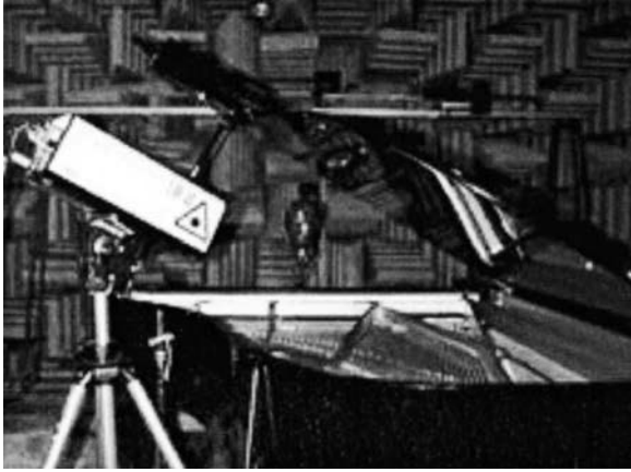
FIG. 8. Experimental setup. The grand piano was isolated in an anechoic room, and both the string vibrations and the acoustical radiated signal were measured. The string vibrations were measured using both an accelerometer located at the bridge level and a laser vibrometer, while the acoustic signal was measured at the head level of the pianist using an artificial headset. Our library of measured data also includes signals corresponding to various hammer velocities [referred to in recent and forthcoming articles concerned with the hammer-string interaction (Ref. 31)], but for this paper, we only need acceleration measurements for each string.
