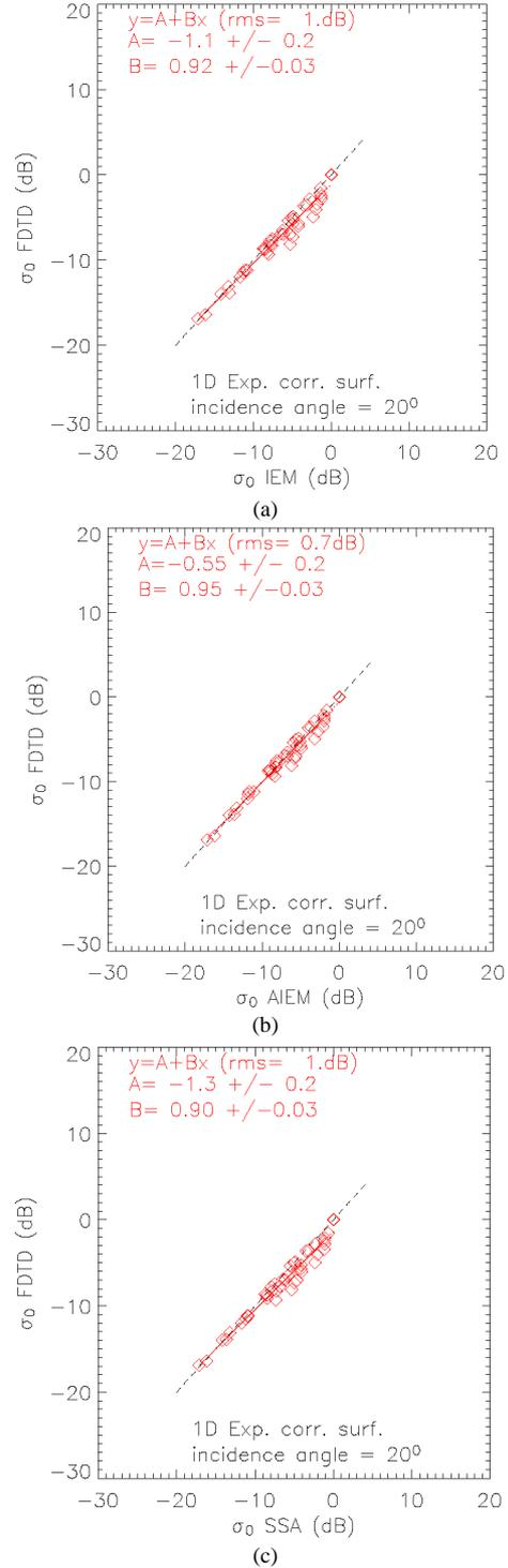
Figure 1: FDTD simulations versus (a) IEM (b) AIEM and (c) SSA predictions at VV polarization and 20° incidence angle. The parameters of a linear fit between FDTD and the asymptotic model values as well as the overall rms error are reported.
