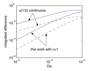
FIGURE 7. Integrated difference in horizontal (continuous line) and vertical (dashed line) velocities between mixed Stokes-Darcy and Darcy-Brinkman results as a function of the Darcy number for  $\chi_f = 0.2$ , using our interfacial condition with c = 1 or a continuous horizontal velocity at z = 1/2.
