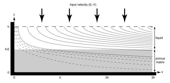
FIGURE 4. Corner flow in a fluid overlying a porous layer with a constant porosity: geometry and streamlines given by the limiting Darcy-Brinkman solution with constant  $\chi_f = 0.2$  and  $Da = 10^{-3}$ . Continuous streamlines are equally spaced from 0.1 to 2.9 with a spacing 0.2, and dashed streamlines from 0.02 to 0.08 with a spacing 0.02.
