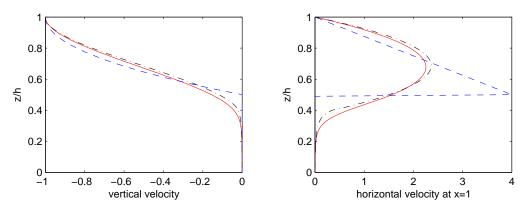
FIGURE 9. Comparison between mixed Stokes-Darcy and Darcy-Brinkman formulations for a corner flow in a fluid overlying a porous layer with a linear porosity ( $Da = 10^{-4}$  and  $\chi_0 = 0.5$ ). Continuous line: Darcy-Brinkman; dashed line: mixed Stokes-Darcy in the limit  $z_{\delta} \to (1/2)^{-}$  (i.e.  $c \to 0$ ); dashed-dotted line: mixed Stokes-Darcy with c = 1.
