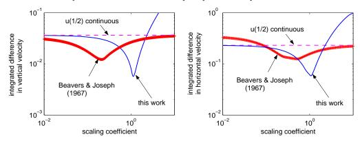
FIGURE 6. Integrated difference between mixed Stokes-Darcy and Darcy-Brinkman results as a function of the scaling coefficient (i.e.  $\alpha$  for Beavers & Joseph (1967) and c for our interfacal conditions) for a corner flow in a fluid overlying a porous layer with a constant porosity ( $Da = 10^{-3}$  and  $\chi_f = 0.2$ ).
