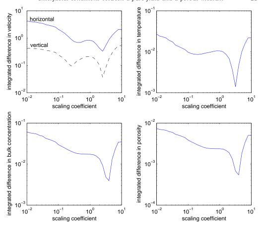
FIGURE 12. Integrated difference between Darcy-Brinkman and mixed Stokes-Darcy formulation with our interfacial conditions as a function of the scaling coefficient c ( $V_{pull}=1$ , V=10, L=10,  $Da=10^{-4}$ ,  $C_e/(C_\infty-C_e)=-7$ , m=0.8).
