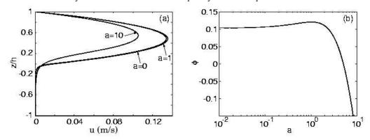
FIGURE 2. (a): Poiseuille flow profiles computed with Darcy-Brinkman formulation for various values of the averaging size  $\delta_a = a\sqrt{\Pi(\chi_f)}$ . (b): relative flow rate increase depending on the scaling coefficient a. In these computations,  $\chi_f = 0.9$ ,  $\Pi(\chi_f)/h^2 = 10^{-3}$  and  $\eta^{-1}dp/dx = -1(m.s)^{-1}$ .
