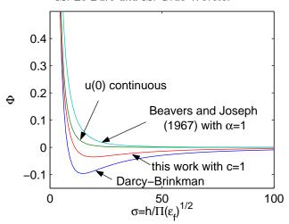
FIGURE 8. Relative flow rate increase as a function of the inverse of the square root of the Darcy number with  $\chi_f = 0.2$ , for the various proposed interfacial boundary conditions. By definition, the condition of zero tangential velocity leads to  $\Phi = 0$ .
