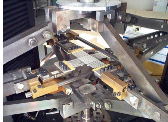
Fig. 3. Biaxial tensile device on cross shape specimens.
