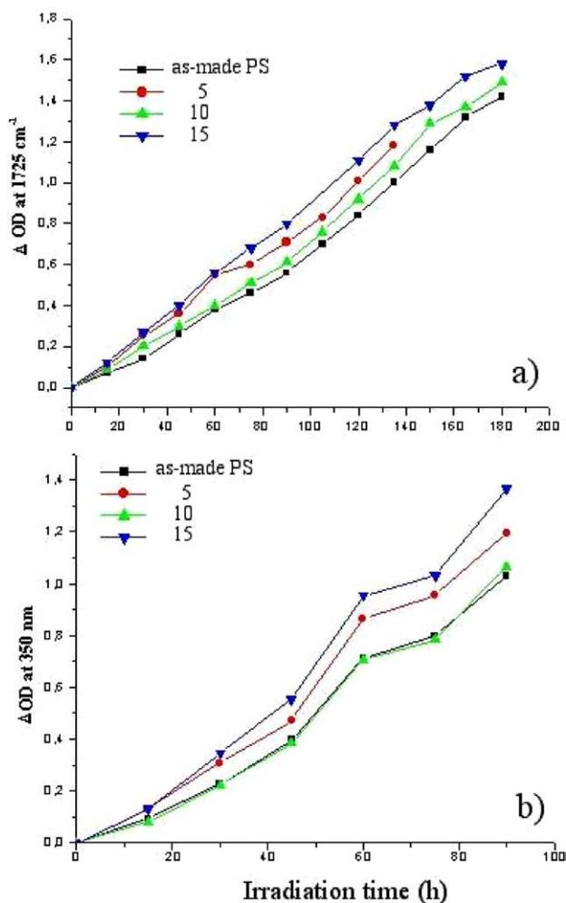
Fig. 11. Variations in (a) IR absorbance at  $1725\text{ cm}^{-1}$ , and (b) in optical absorbance at  $350\text{ nm}$  for the as-made PS and the nanocomposite films SPMA/LDH:PS against irradiation time. The percentage of hybrid LDH is indicated.
