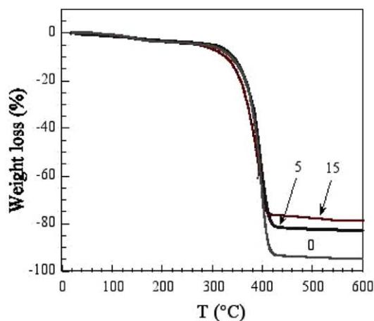
Fig. 7. Thermal analysis of the nanocomposites SPMA/LDH:PS.
