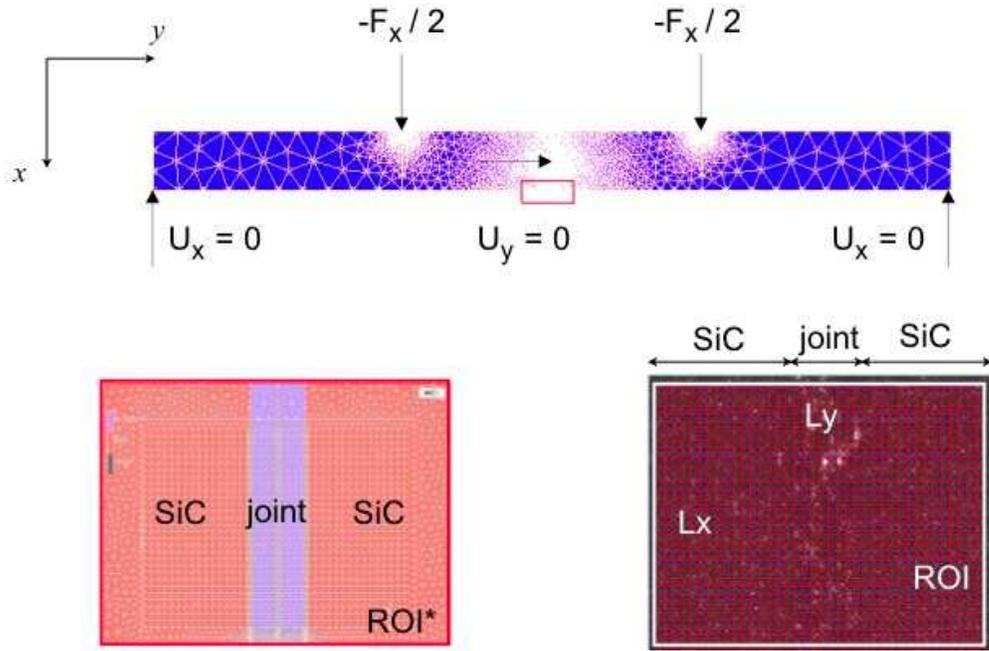
Figure 6. Identification method in four-point bending.
