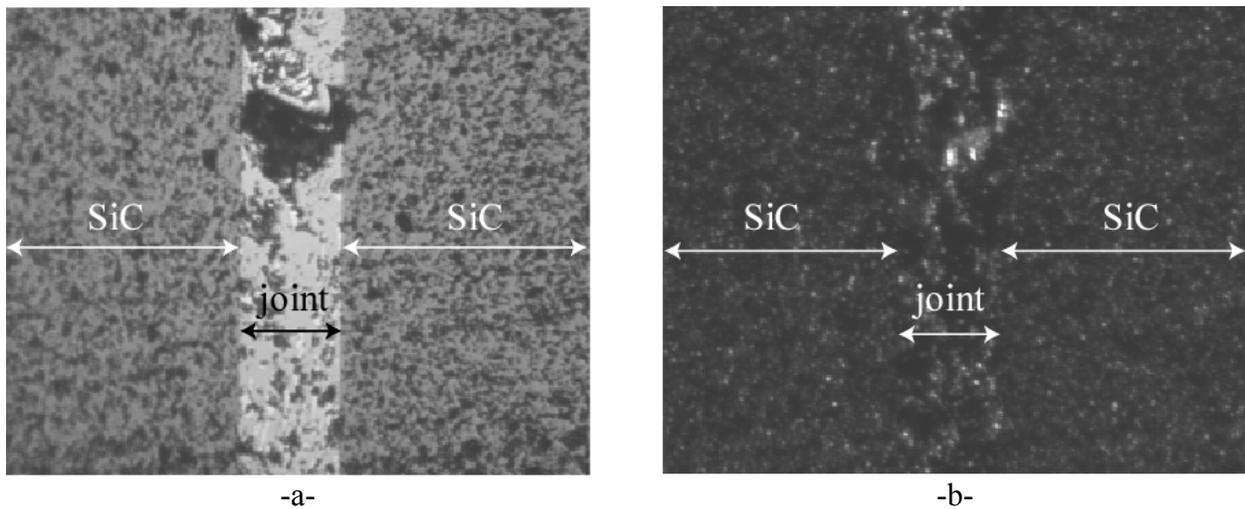
Figure 4. Digital images ( $1280 \times 1024$  pixels, 1 pixel =  $0.33 \mu\text{m}$ ) acquired with a normal lighting beam (a) and a grazing lighting beam (b).
