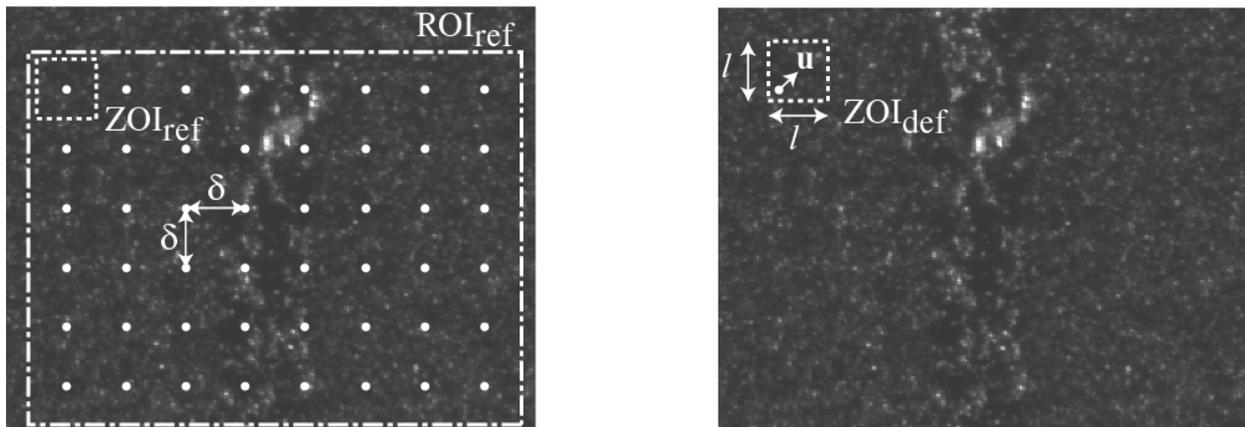
Figure 1. Schematic diagram showing the correlation parameters in a reference picture (left) and a picture in the deformed state (right).
