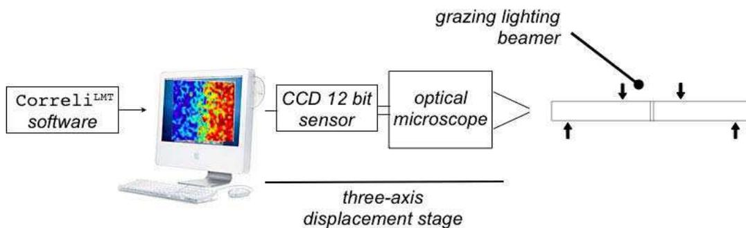
Figure 5. Schematic of the testing procedure using a DIC technique.
