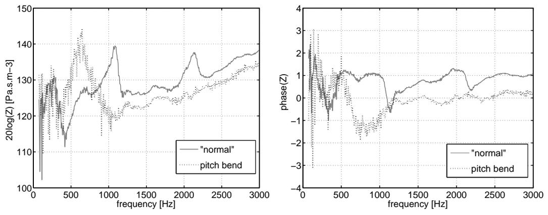
Figure 5: Comparison between the impedance measured for normal playing mode and the one measured for pitch bend
