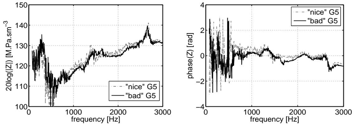
Figure 8: Impedance of a soloist’s vocal tract for two configurations leading either to a “nice” sound or to a “bad” one, which is to be avoided (note G5)
