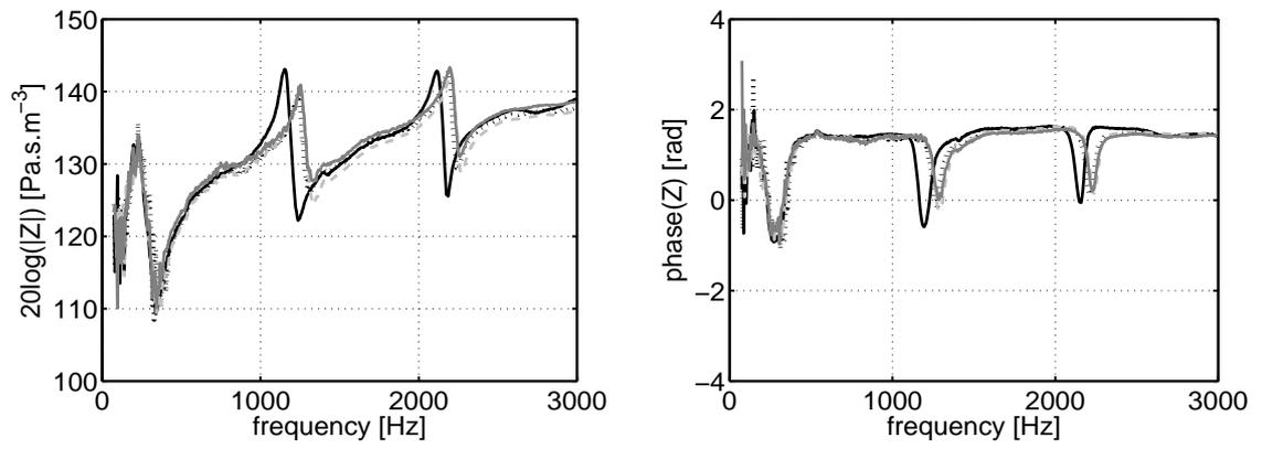
Figure 3: Test of reproducibility : note G3 at different times during 40 minutes
