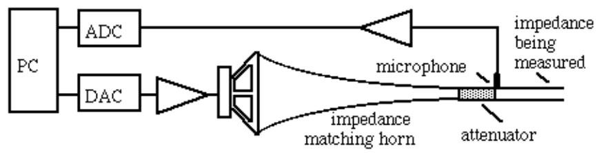
Figure 1: Impedance spectrometer
