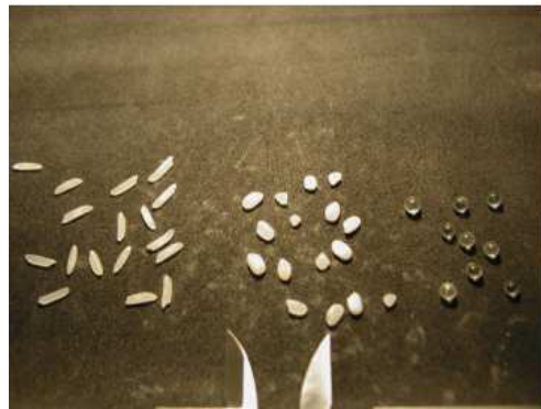
Fig. 2. Picture of the grains used: basmati rice (left), round rice (center) and glass beads (right)
