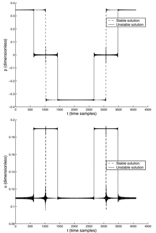
FIG. 15. The pressure (a) and volume-flow (b) wave form of the Helmholtz solution and a 3-level sister solution calculated by the HBM employing the simple clarinet model with  $\zeta = 0.5$ ,  $\gamma = 0.4$ ,  $N_p = 99$ ,  $\eta = 10^{-5}$ .
