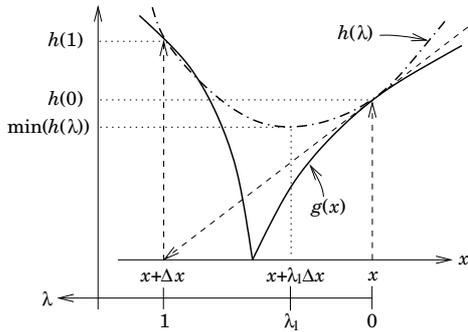
FIG. 6. The principle of backtracking in one dimension. Objective is to estimate the root of  $g(x)$  (solid curve). Broken lines with arrows show how the Newton step  $\Delta x$  from  $x$  leads to divergence.  $h(\lambda)$  (dot-dashed curve) is a 2nd order expansion of  $g(x)$  along the Newton step, i.e. the  $\lambda$  axis. Minimum of  $h(\lambda)$  should be closer to the root of  $g(x)$  than  $g(x + \Delta x)$ .
