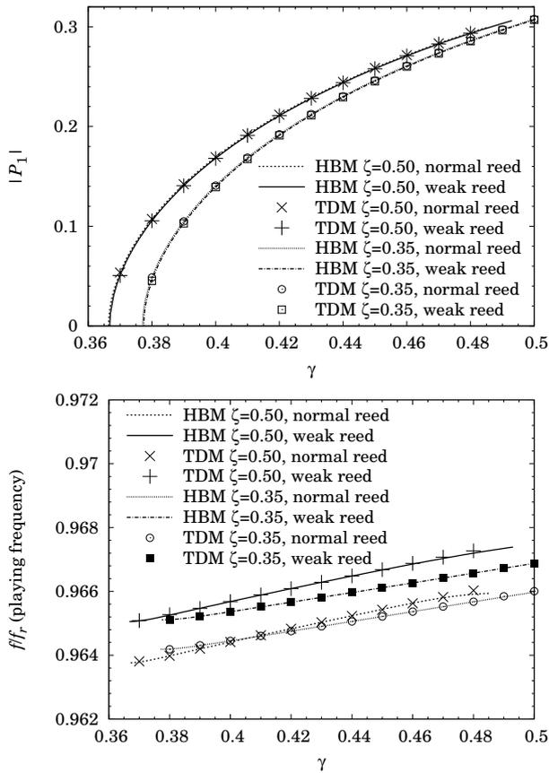
FIG. 14. Comparison between HBM and TDM of the amplitude of (a) the first harmonic  $P_1$  and (b) the dimensionless playing frequency  $f_p/f_r$  as the blowing pressure  $\gamma$  increases for a clarinet-like system with viscous losses and weak and normal reed interaction. TDM values for  $\zeta = 0.50$  and  $\gamma > 0.48$  are omitted due to period doubling. So are the beating regimes of HBM calculations. ( $f_s = 51100\text{Hz}$ ,  $N_t = 512$ ,  $f_r = 103.4\text{Hz}$ ,  $N_p = 15$ )
