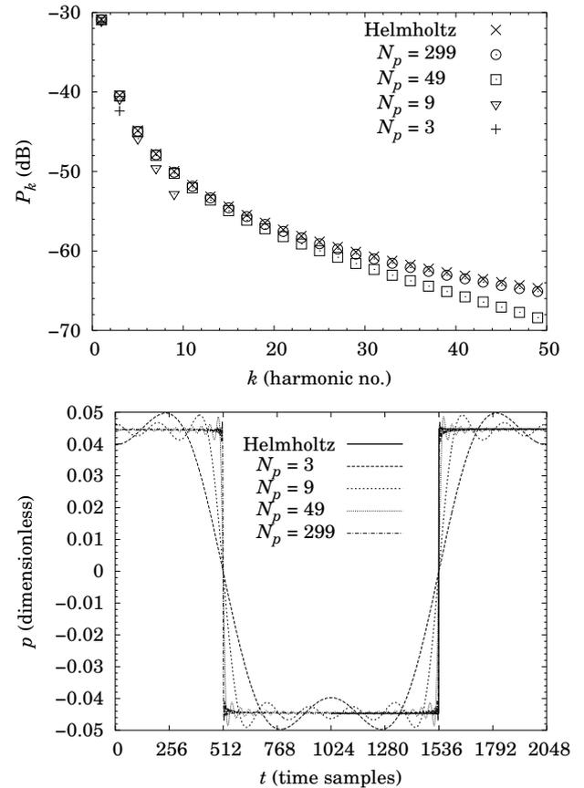
FIG. 8. The Helmholtz solution, eq. (24) compared with the HBM truncated to 3, 9, 49, and 299 harmonics close to the oscillation threshold ( $\gamma = 0.334$ ,  $\zeta = 0.5$ ,  $\eta = 10^{-5}$ ). (a) frequency domain. (b) time domain.
