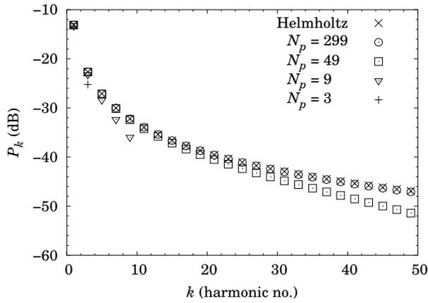
FIG. 9. The Helmholtz solution, eq. (24) compared with the HBM truncated to 3, 9, 49, and 299 harmonics far from the oscillation threshold ( $\gamma = 0.40$ ,  $\zeta = 0.5$ ,  $\eta = 10^{-5}$ ) in the frequency domain.
