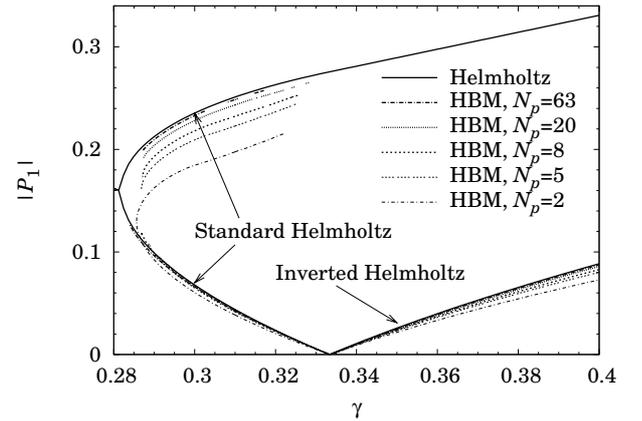
FIG. 13. Amplitude of first harmonic  $P_1$  as a function of the blowing pressure  $\gamma$  for the Helmholtz solution (30) for 2-stepped cone and the HBM truncated to 2, 5, ..., and 63 harmonics, the last coinciding with Helmholtz ( $\zeta = 0.2$ ,  $\eta = 2 \cdot 10^{-5}$ ). Only nonbeating regimes are shown.
