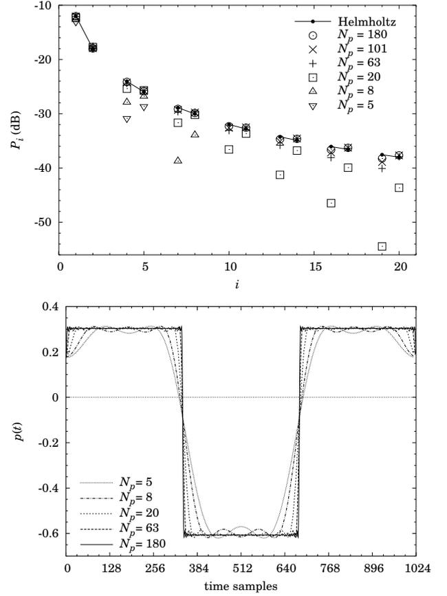
FIG. 12. Comparison between the standard Helmholtz motion of a stepped cone ( $N = 2$ ) and the HBM for various  $N_p$  at  $\gamma = 0.31$ ,  $\zeta = 0.2$ , and  $\eta = 2 \cdot 10^{-5}$ . (a) The magnitude of the harmonics and (b) one oscillation period.  $N_t$  varies from 128 for  $N_p=5$  to 1024 for  $N_p=180$ .
