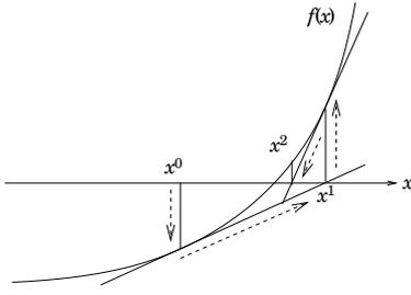
FIG. 1. The iteration process of Newton's method
