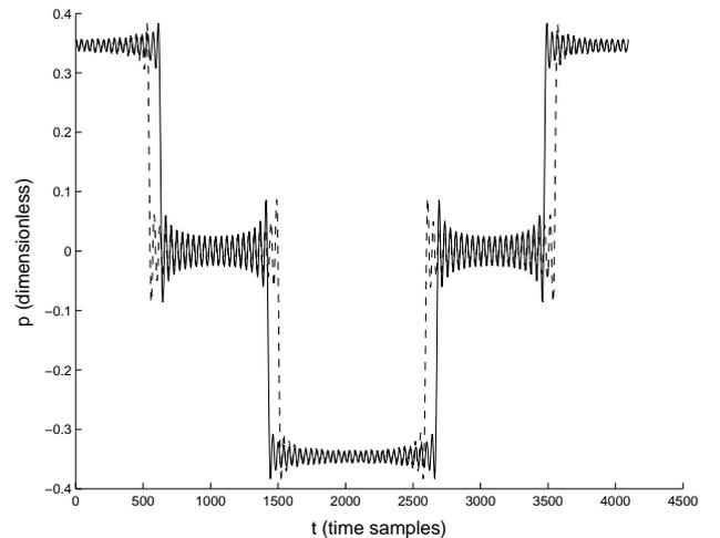
FIG. 17. The pressure waveform of two solutions that differ by the duration of their steps, found by the HBM employing the simple clarinet model with  $\zeta = 0.5$ ,  $\gamma = 0.4$ ,  $\eta = 10^{-5}$ ,  $N_p = 99$ .
