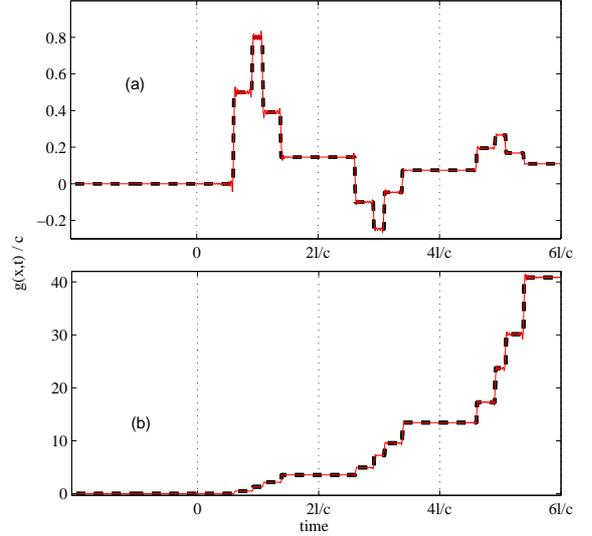
FIG. 2. Normalized Green function as a function of time: comparison between the successive reflections method (dotted line) and modal expansion (solid line, 102 modes, i.e. maximum  $n = 50$ ). Locations of the source and receiver are  $x_0/\ell = 0.15$  and  $x/\ell = 0.76$ , respectively. (a) passive boundaries  $\zeta = 4$ ;  $\zeta_\ell = 0.1$  (constant mode = 0.097). (b) active boundary  $\zeta = \zeta_\ell = -4$ . (constant mode = -2).
