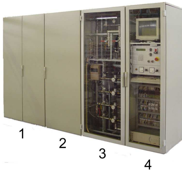
Fig. 8. Power supply source of the three-phase plasma torch (power up to 500 kW)
