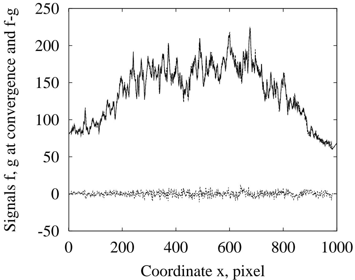
Fig. 6. Superimposed profiles  $f$  (dashed line) and  $g$  (solid line) accounting for the displacement field as determined by using 55 Fourier modes. The bottom curve corresponds to the difference  $f - g$ , i.e., an estimate of the error.
