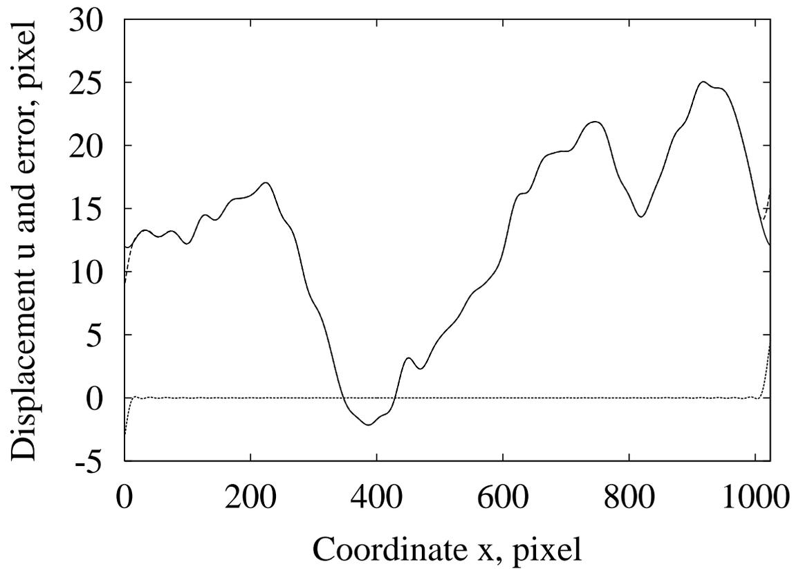
Fig. 3. The solid line shows the prescribed displacement (defined by using 30 Fourier modes), while the dashed line is the estimate obtained from the present method after  $8 + 41$  iterations (i.e., 95 Fourier modes). Note that the only significant error (bottom curve) between the prescribed and computed displacement field is confined on the edges of the signal.
