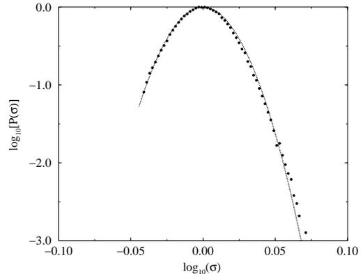
FIG. 8: Surface stress distribution for self-affine surfaces of roughness exponent  $\zeta = 0.8$  and of roughness amplitudes  $A = 0.05\epsilon_{max}$ ,  $\epsilon_{max}$  is the amplitude such that the maximum local slope is equal to 1. The self-affine interfaces have been built with 32 Fourier modes and the results averaged on 1500 surfaces. We can check that the distribution (symbols) is well fitted by a parabola, which shows that the stress is log-normally distributed.
