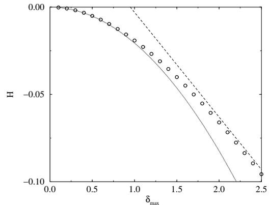
FIG. 5: Shift from the mean plane of the plane equivalent boundary for a Stokes flow in case of self-affine interface of varying amplitude. We use in abscissa the maximum local slope  $\delta_{max}$ . The dotted line correspond to the second order perturbative expansion and the symbols to computations using conformal mapping. The dashed line has a slope -0.06. The surface has been built with 64 Fourier modes and we used 256 modes in the solution based on conformal mapping.
