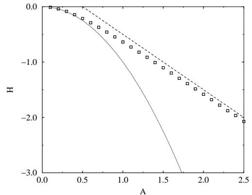
FIG. 4: Shift from the mean plane of the plane equivalent boundary for a Stokes flow in case of sine interface of varying amplitude  $A$ . The dotted line corresponds to the second order perturbative expansion and the symbols to computations using conformal mapping. The dashed line has a slope -1.
