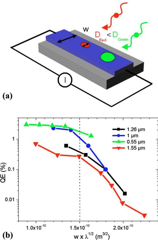
FIG. 1. (Color online) (a) Scheme of the hot-spot. The NbN stripe is in blue (b) Dependence of normalized DE vs reduced parameter  $w\sqrt{\lambda}$  at different wavelengths. This was measured with  $10 \times 10 \mu\text{m}^2$  SSPDs with width varying from 120 to 220 nm.
