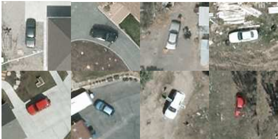
Fig. 6. 100x100 pixels regions centred on cars, extracted from the VeDAI dataset. Small size, specular reflections, shadows or occlusion make the detection challenging.
