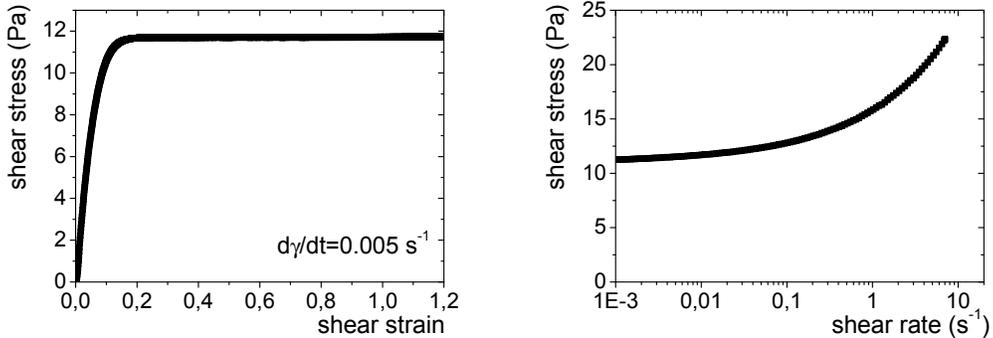
Figure 2: Yield stress measurement (*left*) and flow curve (*right*) of suspending emulsion 2a. The material is elasto-plastic below the yield stress and visco-plastic beyond.
