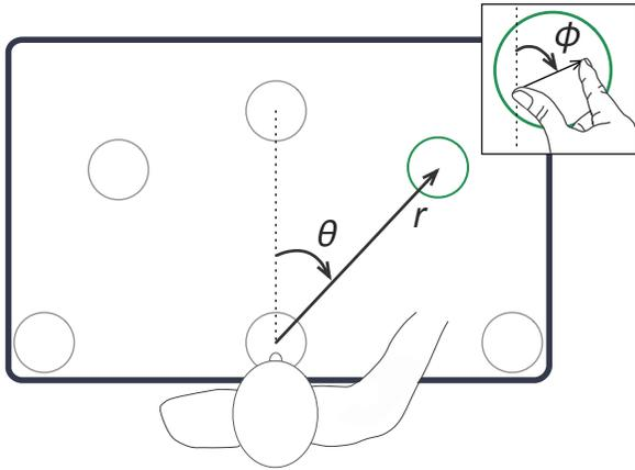
**Figure 2. The position of interactive objects expressed in polar coordinates  $(r, \theta)$ , where  $r$  is the radial distance and  $\theta$  is the clockwise angle with respect to the vertical axis of the screen. The grip orientation is expressed by the clockwise angle  $\phi$  defined by the thumb and the index.**
