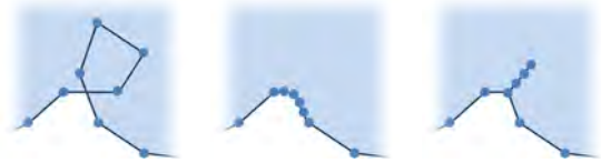
Figure 9. Repairing a self-intersection in a boundary curve (left). Center: moving sample points formerly within the loop onto the intersecting line segment. Right: To reduce stretching, we distribute loop points between the intersection and the loop’s centroid instead.
