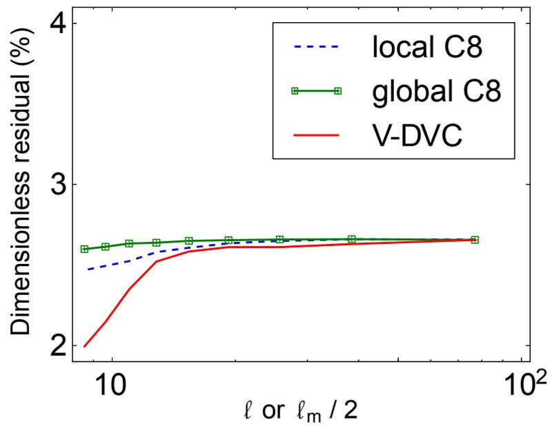
Figure 5: Dimensionless correlation residual vs. element size  $\ell$  or regularization length  $\ell_m/2$  (in voxels).
