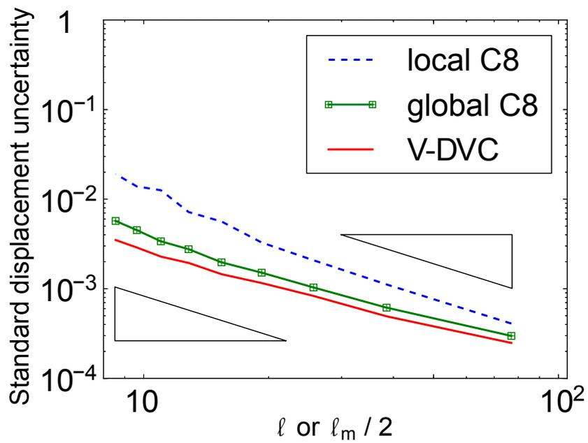
Figure 3: Standard uncertainty of the displacement vs. element size  $l$  or regularization length  $l_m/2$  (in voxels) for a Gaussian white noise ( $\sigma = \sqrt{2}$  gray level). The  $-3/2$  power law dependence is depicted by black triangles.
