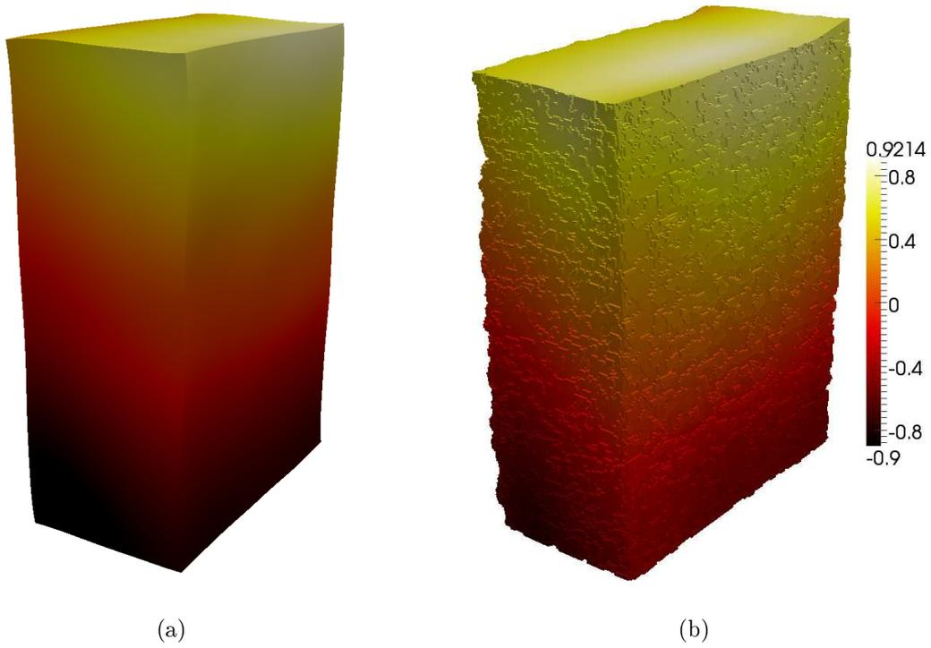
Figure 4: Transverse displacement along the longer edge direction expressed in voxels of the sample described in Section 5 with  $\ell_m = 32$  voxels. Warp factor is equal to 10. The ROI lies inside the sample (a) or contains the outer (lateral) boundaries (b). The size of the analyzed volume is  $100 \times 170 \times 256$  voxels.
