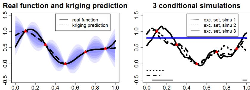
Fig. 1: Conditional simulations of level sets. Left: Kriging model obtained from five evaluations of a  $1d$  function. Right: Three GP conditional simulations, leading to three different level sets. Here the threshold is fixed to  $T = 0.8$ .
