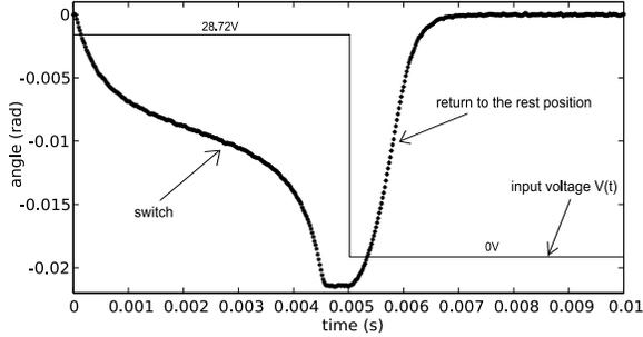
(b)  $V = 28.72 \text{ V} > V_{\text{pullin}}^{\text{dyn}}$
