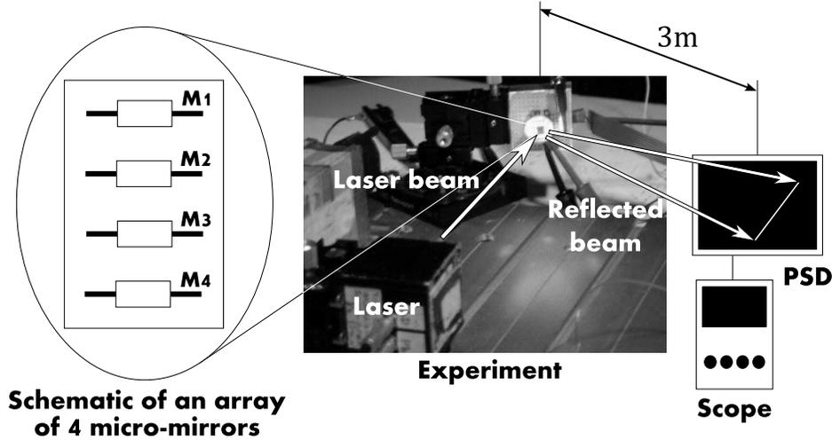
Figure 8: Experimental setup
