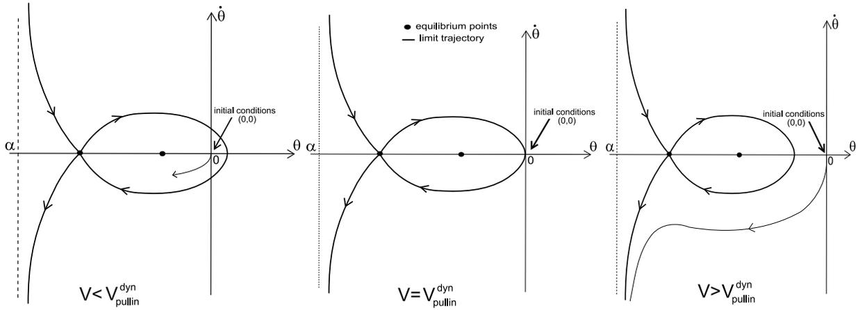
Figure 19: Trajectories according to the value of  $V < V_{\text{pullin}}$ .
