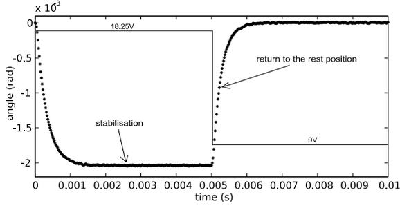
(a)  $V = 18.25 \text{ V} < V_{\text{pullin}}^{\text{dyn}}$
