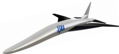
Figure 12: Experimental supersonic airplane model (unmanned aircraft with no engine and capable of autonomous flight) to be used in D-SEND#2.
