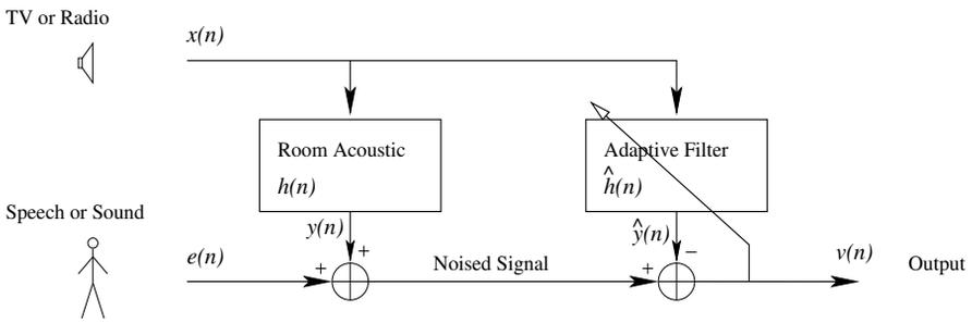
Figure 2: Block diagram of an echo cancellation system
