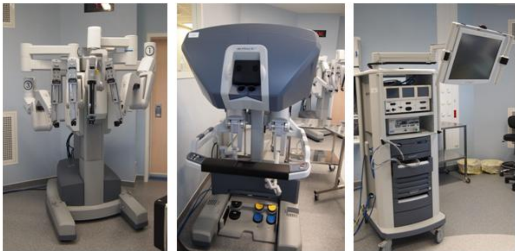
Fig. 1 The da Vinci surgical system, showing (from left to right) the patient cart, console, and tower
