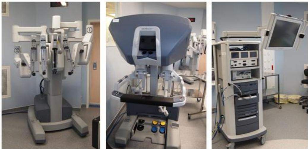
**Fig. 1** The da Vinci surgical system, showing (from left to right) the patient cart, console, and tower
