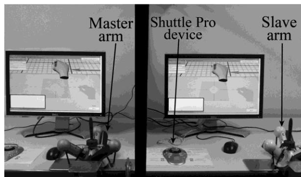
Fig. 5: The haptic communication system with two haptic arms
