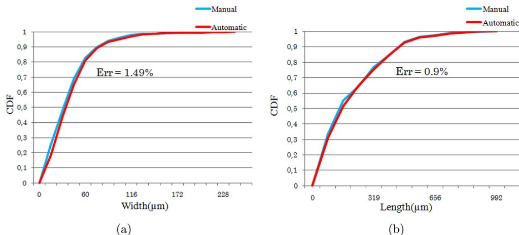
**Figure 6.** Comparison of cumulative distribution functions (CDF) of particles length and width for 150 in-situ images. (a) Comparison of particles width distributions. (b). Comparison of particles length distributions.
