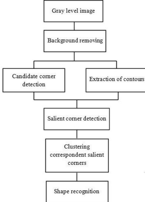
**Figure 2.** The diagram of the proposed method
