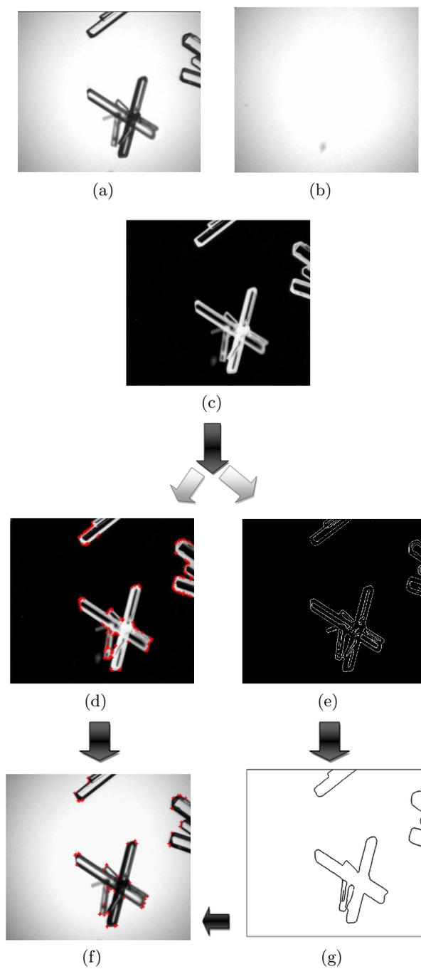
**Figure 3.** Example of the salient corner detection applied on a real image of Ammonium Oxalate crystals. (a) Original gray level image. (b) Background image. (c) Removing the background from image (a). (d) Candidate corners image. (e) Multi-scale edge detection. (f) Edge image after contour completion and edge cleaning steps. (g) Salient corners image.
