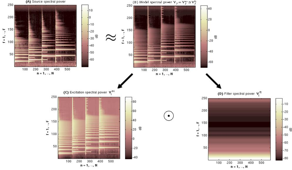
Fig. 3. Excitation-filter decomposition as applied to the spectral power of several guitar notes. (A): source spectral power, (B): model spectral power  $V_j = V_j^{ex} \odot V_j^{ft}$ , (C): excitation spectral power  $V_j^{ex}$ , (D): filter spectral power  $V_j^{ft}$ .
