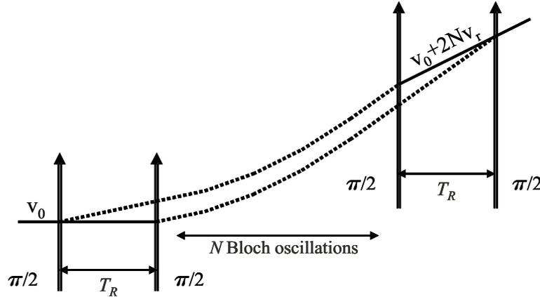
Figure 2: Scheme of the interferometer used for the measurement of  $h/m_{\text{Rb}}$ . The first pair of  $\pi/2$  pulses produces a fringe pattern in the atomic velocity distribution which is measured by the second pair of  $\pi/2$  pulses. Between these two pairs of pulses, the atoms are accelerated upwards or downwards. The solid line corresponds to the atom in the  $F = 2$  state, and the dashed line to the  $F = 1$  state.
