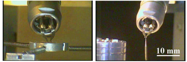
Fig. 5. axis calibration of a compliant table and tool transform calibration.
