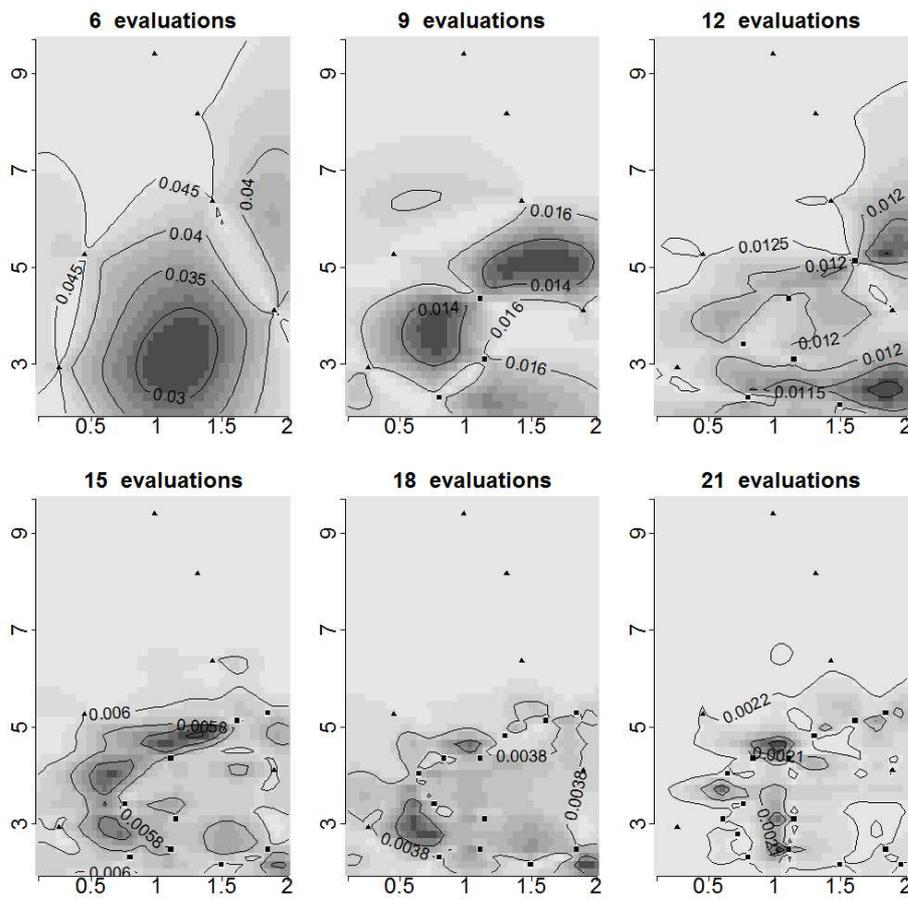
**Fig. 6** Plot of the value of the criterion  $J_n^{(\Gamma)}(x) = \mathbb{E}_n \left( \int_{\mathbb{X}} p_{n+1}(1 - p_{n+1}) d\mathbb{P}_{\mathbb{X}} \right)$  after  $n$  evaluations of the MORET code. At each iteration, the point chosen for sampling is the optimum of this function. Areas in black correspond to potentially interesting areas, where the uncertainty  $H_n^{(\Gamma)}$  is reduced the most in expectation.
