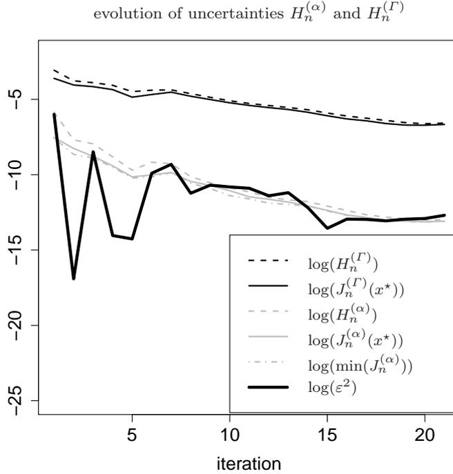
**Fig. 3** Evolution of  $H_n^{(\Gamma)}$  and  $H_n^{(\alpha)}$  during the inversion. The optimum  $J_n^{(\Gamma)}(x^*)$  of the  $J_n^{(\Gamma)}$  criterion is usually lower than  $H_n^{(\Gamma)}$  and corresponds to the expectation of  $H_n^{(\Gamma)}$  at the next iteration. Regarding the  $J_n^{(\alpha)}$  criterion, the curves  $\min(J_n^{(\alpha)})$  and  $J_n^{(\alpha)}(x^*)$  coincide only when  $x^*$  is also the minimizer of  $J_n^{(\alpha)}$ .
