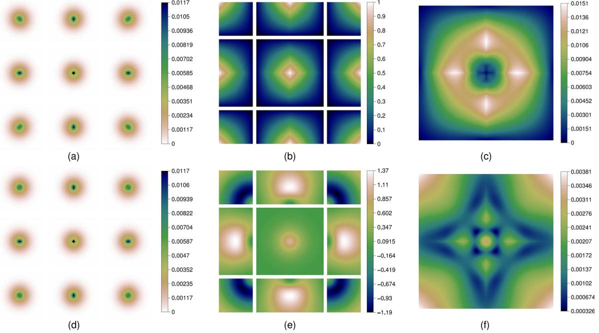
**Fig. 2.** PSF approximation: (a)-(c) using bilinear interpolation; (d)-(f) generalized interpolation with optimal PSF and weights; (a), (d): PSF grid; (b), (e): interpolation weights on each of the 9 patches; (c), (f): rms error with respect to target PSF.
