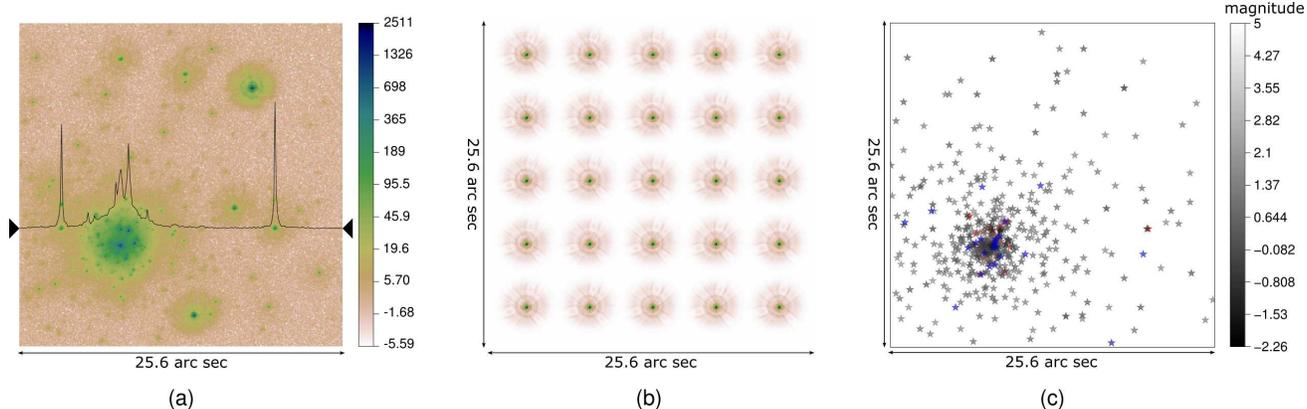
**Fig. 3.** Deconvolution with shift-variant PSF: (a) simulation of an observation of a star field with Hubble’s Wide Field Camera before corrective optics; (b) provided  $5 \times 5$  grid of PSF; (c) recovered stars after deconvolution with sparsity prior, gray: good detection, blue: non-detected star (4.9%), red: false-detection (7.2%)
