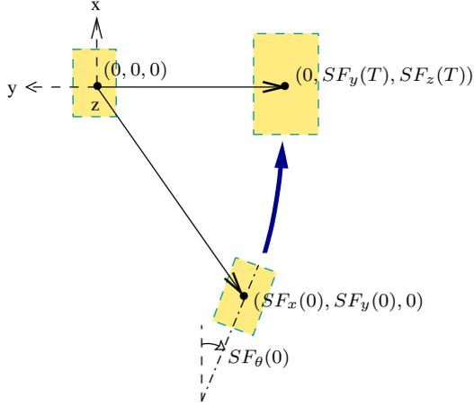
Fig. 1. Here we show an upward half-step from above. It is fully determined by the 5 parameters  $SF_x(0)$ ,  $SF_y(0)$ ,  $SF_\theta(0)$ ,  $SF_y(T)$  and  $SF_z(T)$ . A downward half-step is also fully determined by 5 parameters.
