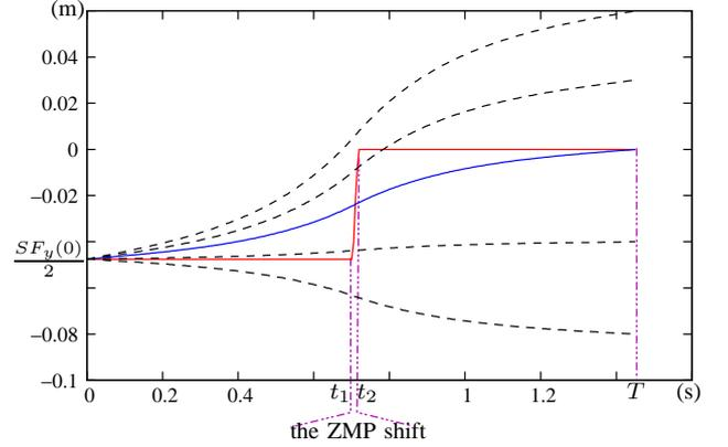
Fig. 2. We consider the upward half-step of Fig. 1, and show in red the corresponding  $p_y(t)$ . To this trajectory correspond an infinity of  $C^2$  solutions for  $y(t)$  which all verify  $y(0) = p_y(0) = \frac{SF_y(0)}{2}$ , each of them being fully defined by  $\dot{y}(0)$ . We show several such  $C^2$  solutions; the curve in blue is the solution retained: it is the unique one verifying  $y(T) = 0$ .
