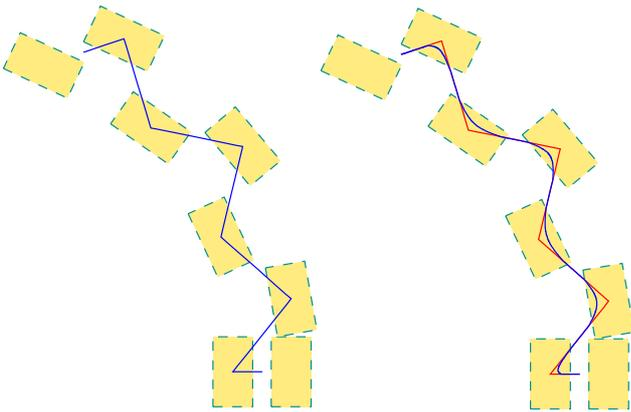
Fig. 4. We illustrate the "smoothing" of a raw sequence of half-steps. On the initial raw sequence (on the left) we can see that the time-free ZMP and CoM trajectories are superimposed. Then, after adjusting the overlaps, the ZMP support path stays the same but the CoM support path becomes smoother (on the right, ZMP in red and CoM in blue).
