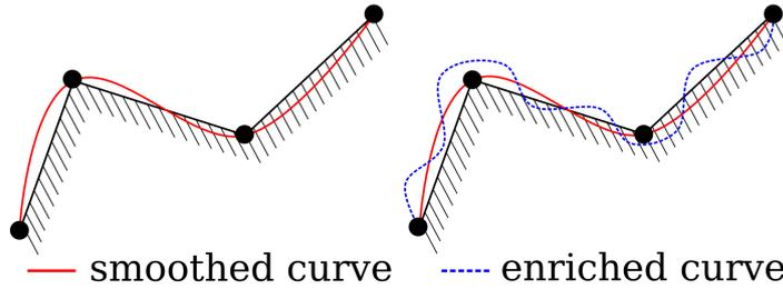
FIG. 2 – Enriched geometry of the smoothed master surface.
