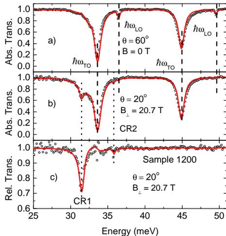
FIG. 1: Experimental transmission spectra (empty dots) of sample 1200. a) absolute transmission for  $B = 0 T$  and  $\theta = 60^\circ$ ; b) and c) absolute transmission and relative transmission respectively for  $B_\perp = 20.7 T$  and  $\theta = 20^\circ$ . The continuous red curves are the fit of data with the model described in the text.
