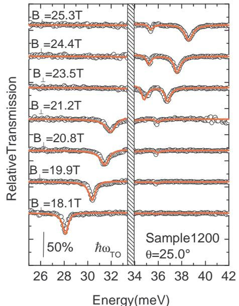
FIG. 3: Fit of the relative transmission curves for sample 1200 at  $\theta = 25^\circ$ . The curves are shifted for clarity. Empty dots are experimental points and full continuous curves the corresponding calculated relative transmission spectra. The hatched region corresponds to that of  $\hbar\omega_{TO}$  (GaAs) (see text).
