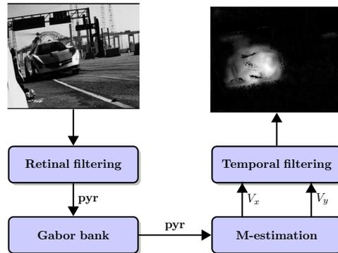
**Figure 2. Block diagram for partitioned dynamic pathway**
