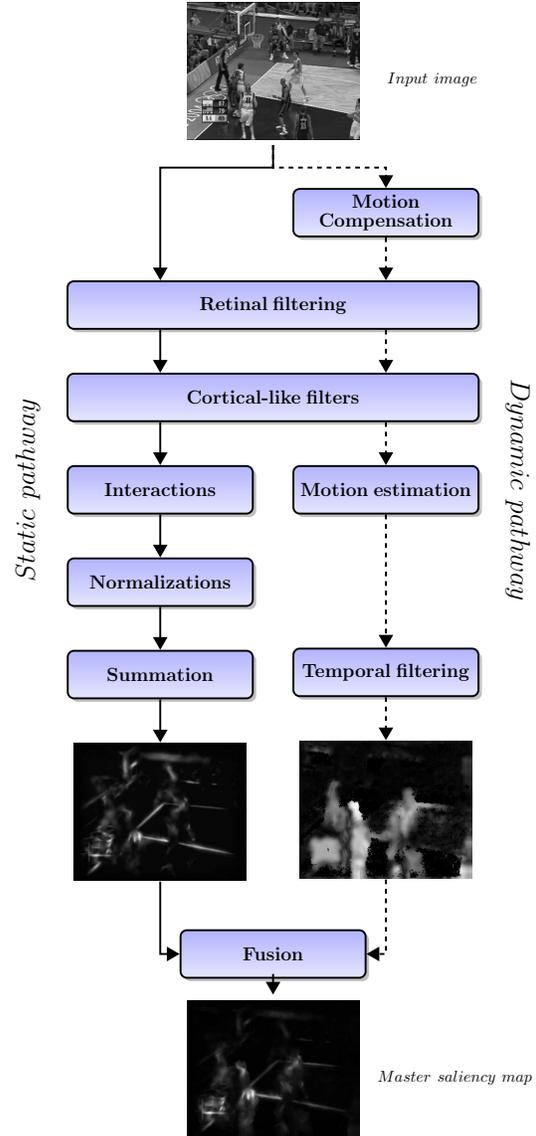
**Figure 1. Block diagram of spatio-temporal visual saliency model**
