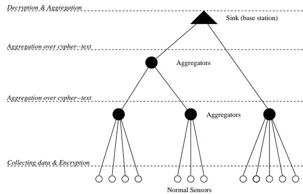
Fig. 1.1. Secure data aggregation in sensor networks
