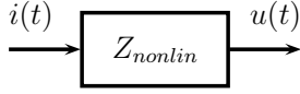
Figure 2: Nonlinear relation between current i(t) and voltage u(t) expressed as a general nonlinear system.
