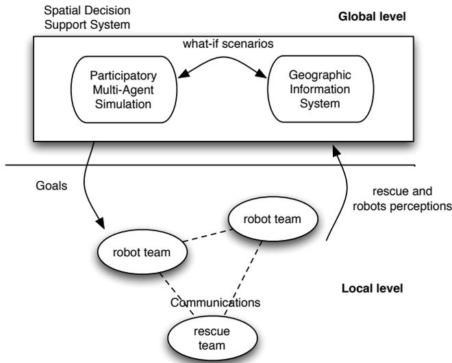
Fig. 1. Functional architecture of the AROUND project
