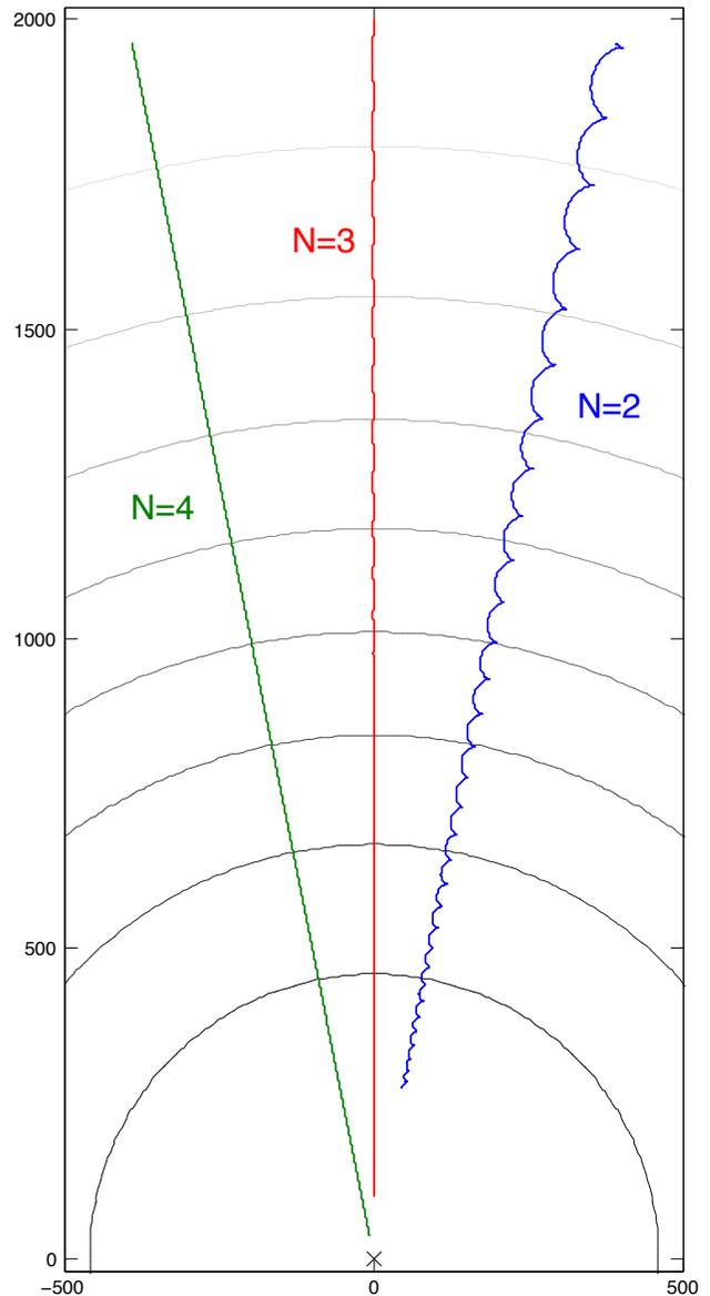
Fig. 3. Trajectories of the formation center  $\mathbf{c}_d$  for different numbers of agents  $N$  when  $\rho$  has circular level sets. For this simulation  $\rho(\mathbf{z}) = e^{-5 \times 10^{-7} \mathbf{z}^\top \mathbf{z}}$ ,  $R = 200\text{m}$ , and  $\omega = 0.01 \text{ rad/s}$ . Location of source is denoted by the  $\times$ .
