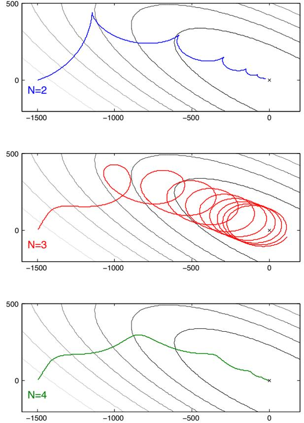
Fig. 6. Trajectories of the formation center  $c_d$  for different numbers of agents  $N$  when  $\rho$  has elliptical level sets. For this simulation the signal function was given by (34),  $R = 1000\text{m}$ , and  $\omega = 0.002 \text{ rad/s}$ . Location of source is denoted by the  $\times$ .
