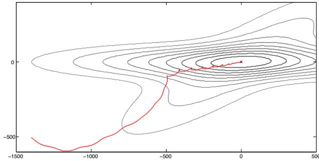
Fig. 8. Trajectories of the formation center  $c_d$  when  $\rho$  is the sum of two gaussian functions (and does not meet the conditions of the theorems). For this simulation  $N = 4$ ,  $R = 200\text{m}$ , and  $\omega = 0.01 \text{ rad/s}$ . Location of source is denoted by the  $\times$ .
