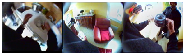
Fig 2a. Motion blur due to strong motion. Fig 2b. High lighting while facing a window. Fig 2c. High lighting while facing a window.
