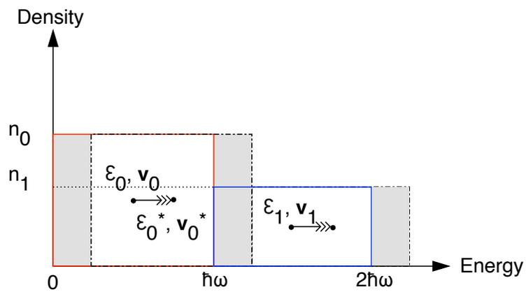
Figure 2: Principle of the computation of the new densities to take heating into account. The red and blue rectangles represent the two initial groups corresponding to energies  $\epsilon_0$  and  $\epsilon_1$ . After heating, these two groups are shifted and have to be projected to compute the new densities of each energy level. We assume that the electrons are uniformly distributed in each group.
