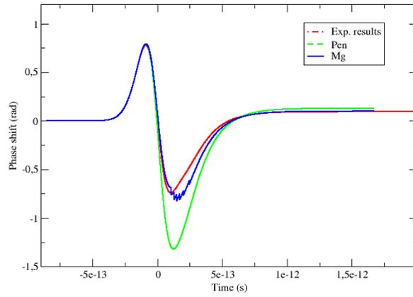
Figure 15: Phase shift (in rad) in  $\text{SiO}_2$  for the three approaches for an intensity of  $2.1 \text{ TW}/\text{cm}^2$ . "Pen" denotes the curve obtained with the temperature model [16], "Mg" the curve obtained with the multigroup model described in this paper and "Exp. results" the results from [14].
