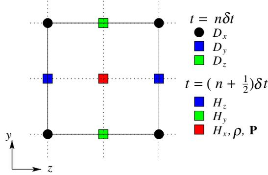
Figure 3: Scheme used to discretize the physical variables.
