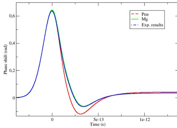
Figure 14: Phase shift (in rad) in  $\text{SiO}_2$  for the three approaches for an intensity of  $1.4 \text{ TW}/\text{cm}^2$ . "Pen" denotes the curve obtained with the temperature model [16], "Mg" the curve obtained with the multigroup model described in this paper and "Exp. results" the results from [14].
