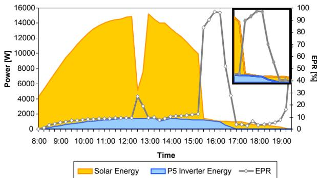
Figure 7 : Energy production and EPR evolution of P5 plant with BL topology on April 3rd 2009
