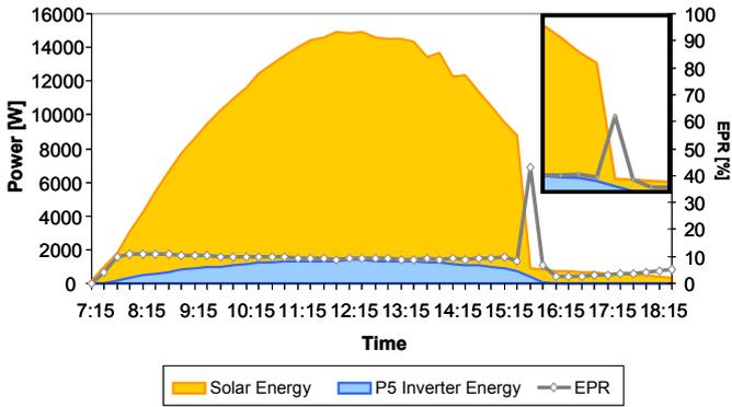
Figure 5 : Energy production and EPR evolution of P5 plant with SP topology on March 20th 2009
