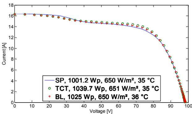
Figure 4 : Current-voltage characteristic of measurements with artificial static shading in 4-5 configuration
