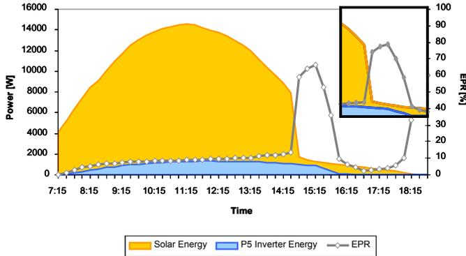
Figure 6 : Energy production and EPR evolution of P5 plant with TCT topology on March 25th 2009
