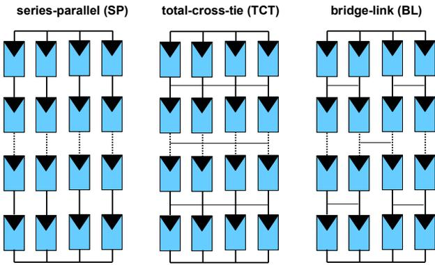
Figure 2 : Diagram showing series-parallel, total-cross-tie, and bridge-link array topologies
