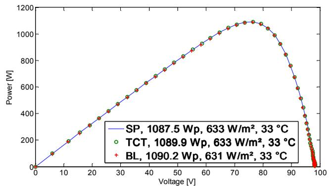
Figure 3 : Power-voltage characteristic carried out in 4-5 configuration normal operating conditions
