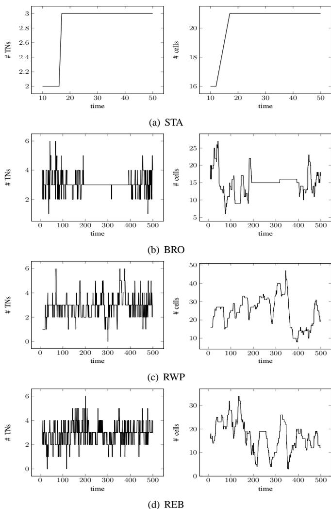
Fig. 7. Evolution of the cover and zone numbers over time for a specific IN. In this simulation, we consider 80 INs and a simulation time of 500s. Optimal value of TNs per IN is  $\sim 3$  and average value of Cells per IN is  $\sim 16$ .
