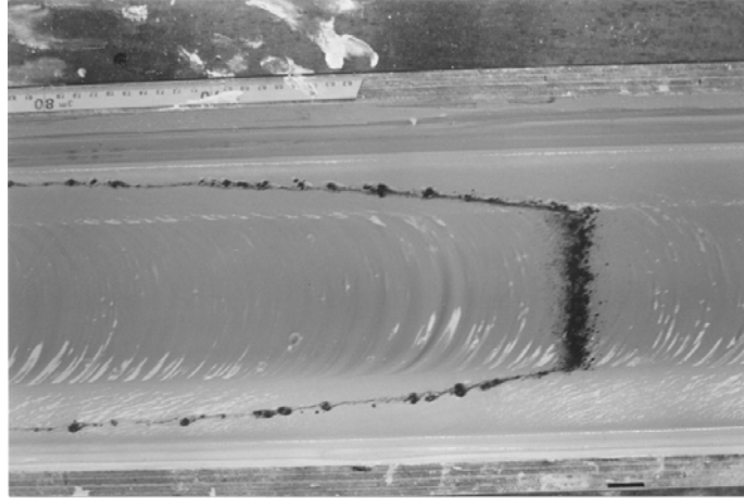
Figure 2 : View from above of the free surface of a kaolin suspension flowing (here from left to right) in steady-state in an inclined, rectangular, open channel. A pepper line was dropped upstream perpendicularly to the flow direction. It now appears deformed due to the shear along the walls, and undeformed in the central plug region. Remark that the slight “dunes” at the free surface were formed far upstream at the hopper exit and do not play any role. [reproduced with Courtesy from APS, Coussot et al. 2002a]
