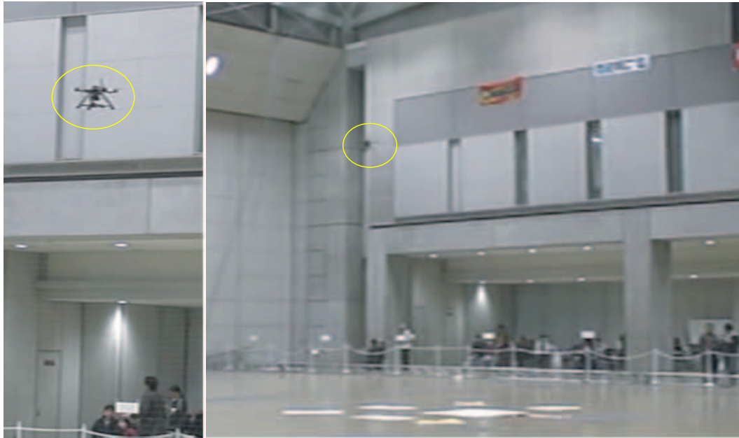
Fig. 11. Indoor fully autonomous flight using optic flow. Demonstration at Tokyo Big Sight for an international exhibition.
