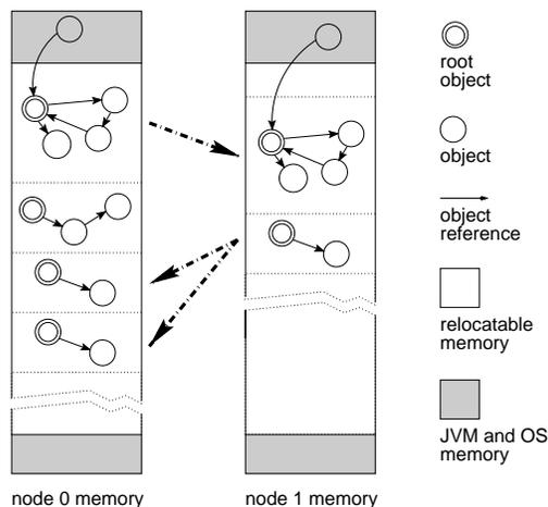
**Figure 2. Relocatable memory for a two-node network**
