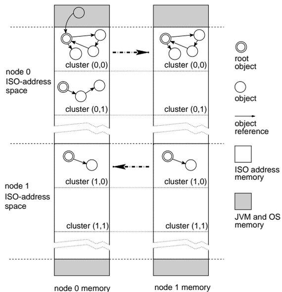
**Figure 1. ISO-address memory for a two-node network**
