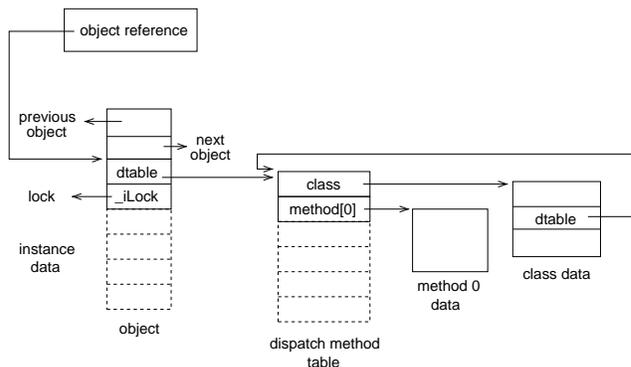
**Figure 4. Object structure in the Kaffe virtual machine**
