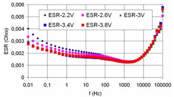
Fig. 8 : ESR v. frequency for different voltages
