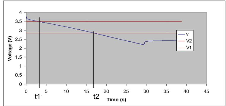
Fig. 4: Li-ion capacitor discharge at constant current
