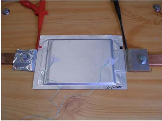
Fig. 2: Lithium Ion capacitor
