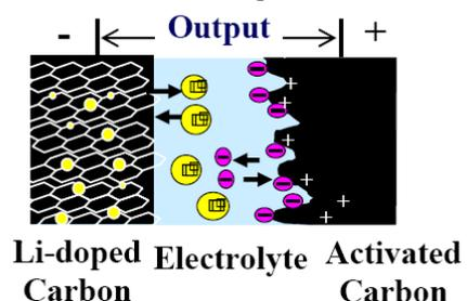
Fig. 1: Elementary structure of EDLC and Li-ion capacitor (JM Energy [1])
