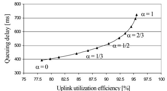
**Figure 6 : Delay vs. Efficiency**
