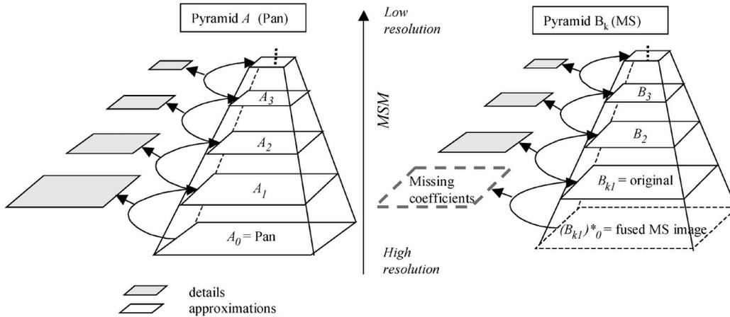
Fig. 8. Hierarchical decomposition of the information (ARSIS concept).
