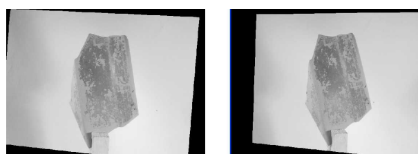
Figure 4: The two images resampled in epipolar geometry
